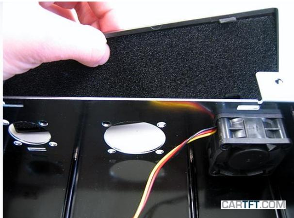
Now the case ventilator is placed from the outside...into the middle:
