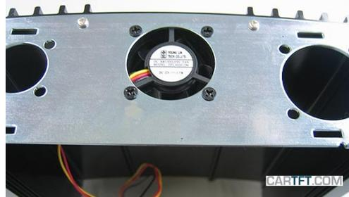
The floor metal gets pushed into the case carefully, so that no cable gets stuck and damaged. The case ventilator cable has to be carried to be in the position to be attached soon
