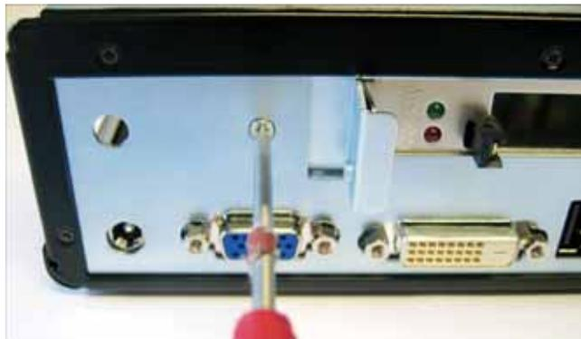
7. Afterwards, connect (screw) the PCI card with the angle bracket.
