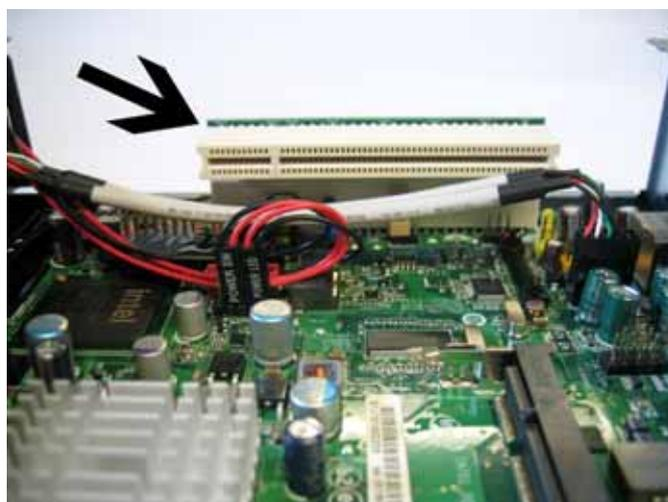
4. Plug the chosen PCI card in to the PCI slot of the Riser card and make sure that the nose attached to the PCI card is fastened at the dedicated spot of the I/O panel (on the left hand side as seen from inside).
