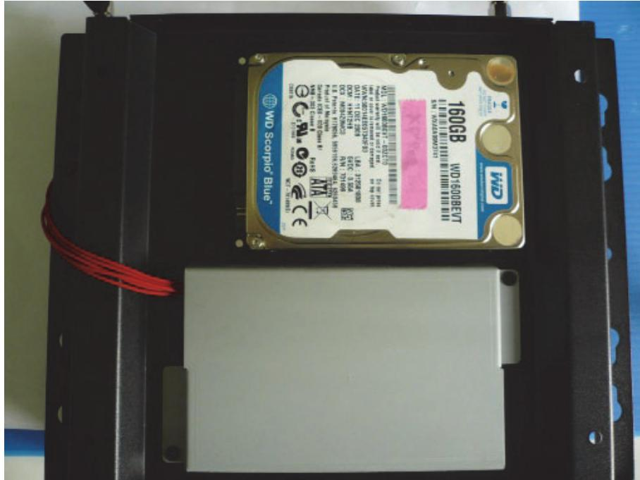
**Step 2.** Turn over the Back Cover and screw the four screws of the Back Cover as shown in the picture.
