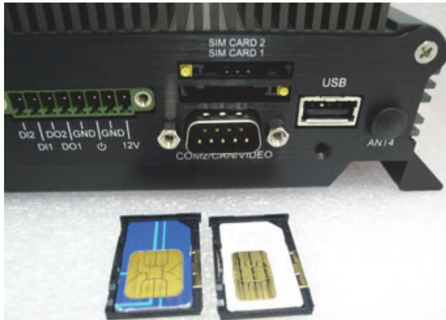
**Step 4.** Take the SIM card holder and Insert it into the socket as shown in the picture.
