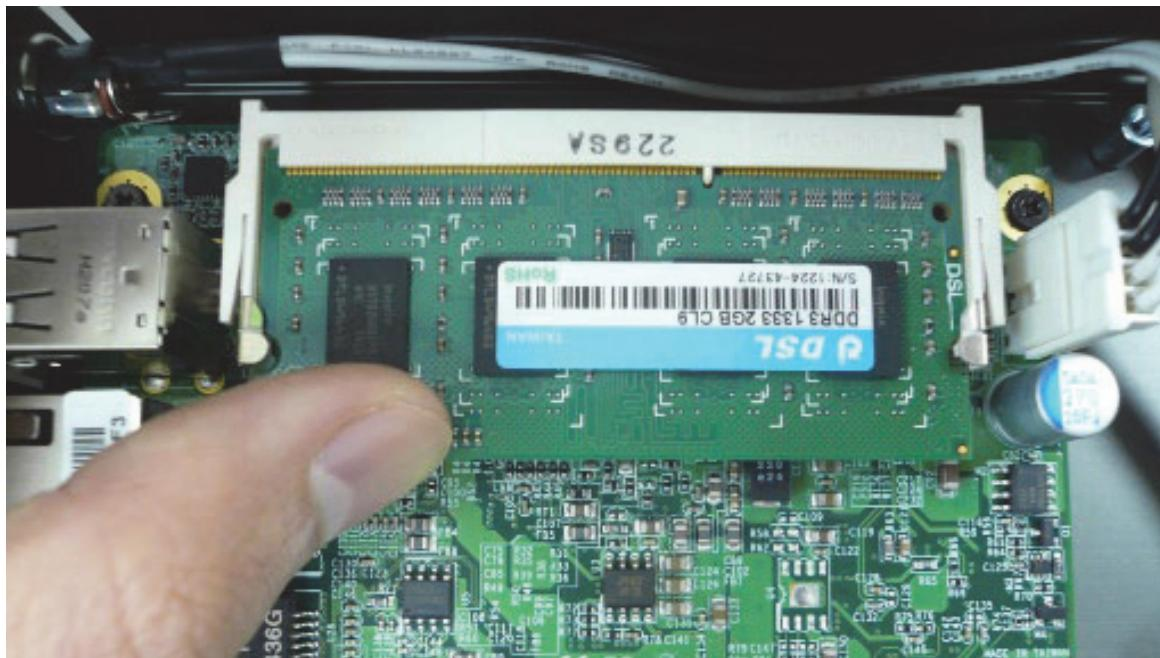
**Step 4.** Press down on the Memory so that the tabs of the socket lock on both sides of the module.
