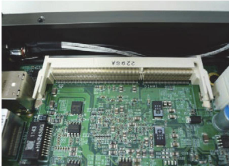
**Step 2.** Hold the Memory with its notch aligned with the Memory socket of the board and insert it at a 30-degree angle into the socket as shown in the picture.
