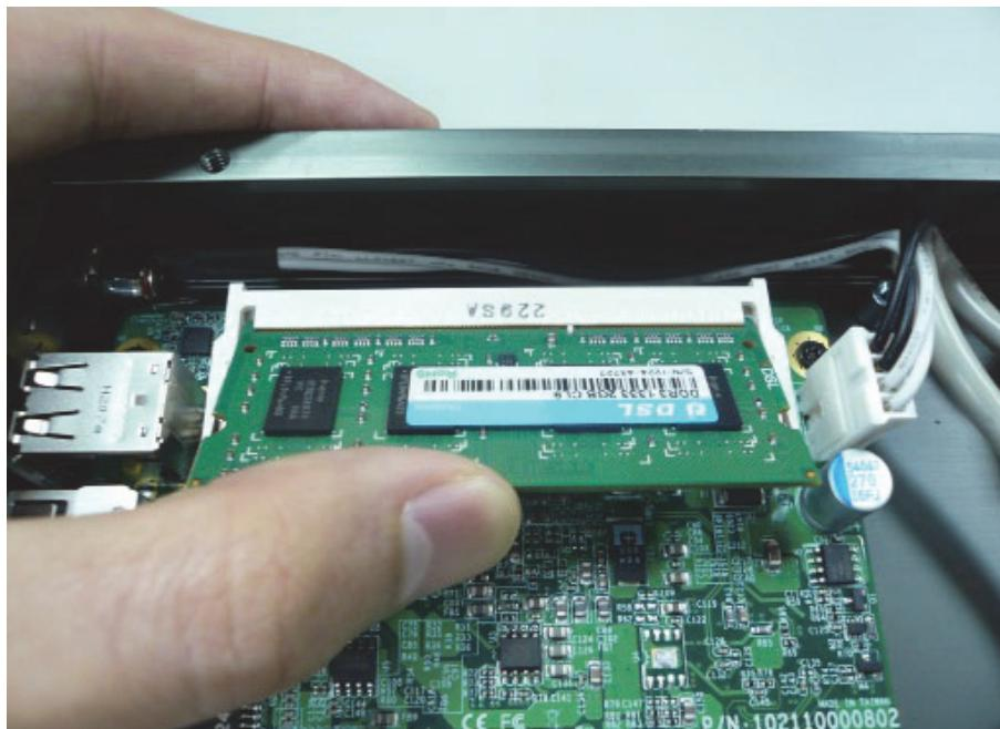
**Step 3.** Fully insert the module into the socket until a “click” is heard as shown in the picture.
