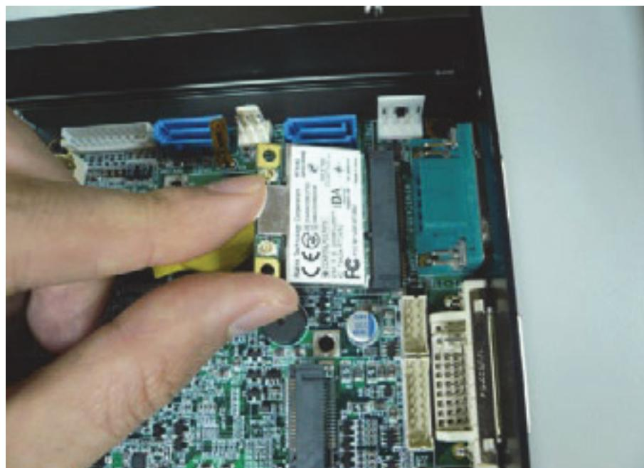
**Step 3.** Screw two screws to the holder as shown in the picture.
